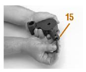
16. Remove relief valve from housing bore.
