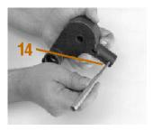
15. The relief valve spring can now be removed from relief valve housing bore.
