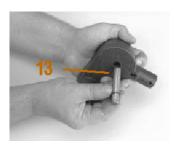
14. Remove relief valve roll pin from pump housing.
