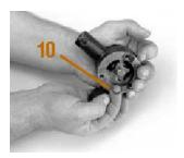
11. Remove internal oil pump element from drive shaft.
