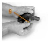
10. Remove element snap ring from drive shaft.
