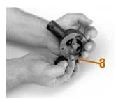
9. Install drive gear key in keyway of drive shaft.
