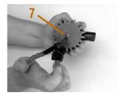
8. Remove drive gear from pump drive shaft.
