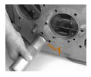
2. Install relief valve in integral oil pump housing.
