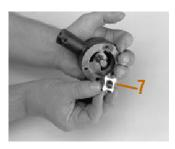
8. Install inner element retention snap ring in drive shaft snap ring groove.
