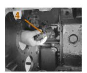
5. Remove integral oil pump retainer plate from case.
