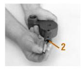
3. Install relief valve spring in oil pump housing.
