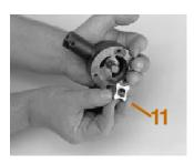
12. Remove two keys from drive shaft keyways.
