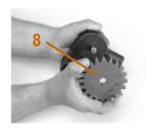
9. Remove key from drive shaft keyway.
