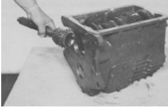
Figure 7 - Remove main drive gear and bearing assembly.
