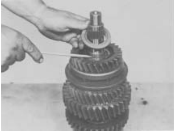
Figure 25 - Remove washer and lock ball.
