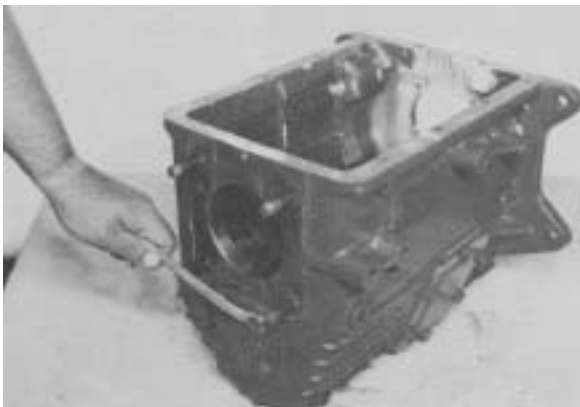
Figure 9 - Remove countershaft bearing cap bolts.
