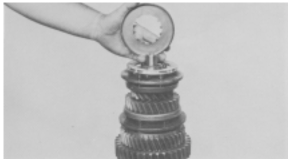
Figure 18 - Remove 5th-Speed synchronizer cup.
