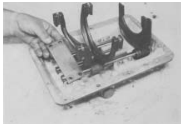
Figure 83 - Position front rail support over shift rails and install cap screws. Position rear support over rails and install cap screws.
