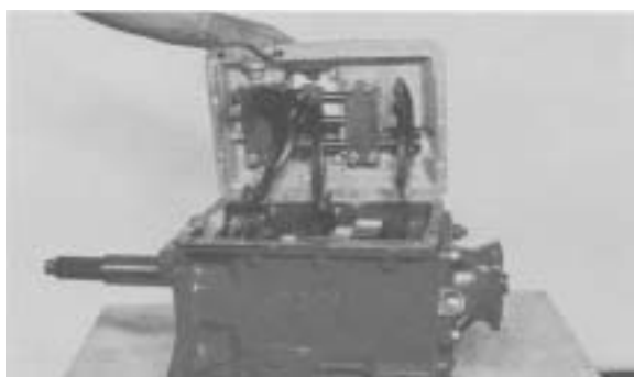
Figure 2 - Remove control cover assembly.
