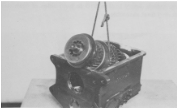
Figure 97 - Position mainshaft assembly in transmission as shown.
