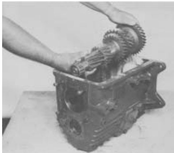
Figure 12 - Remove countershaft assembly.
