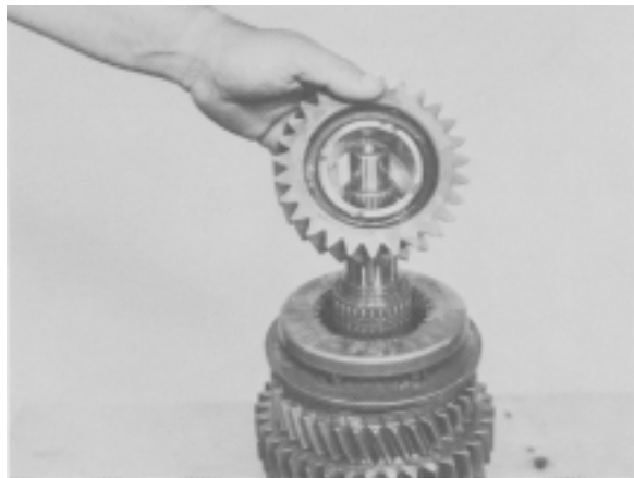
Figure 26 - Remove 3rd speed gear.
