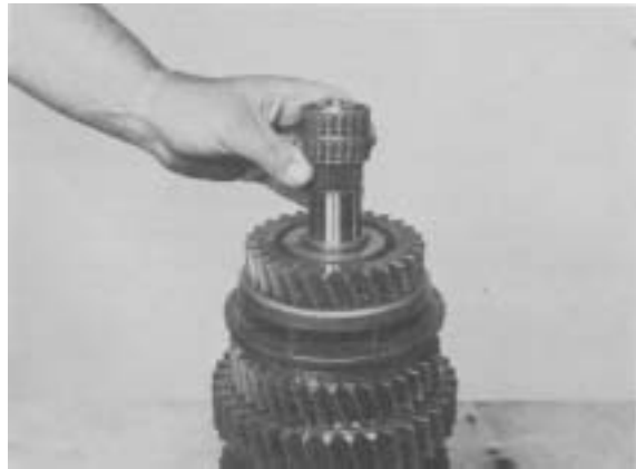
Figure 23 - Remove 4th gear bearing.
