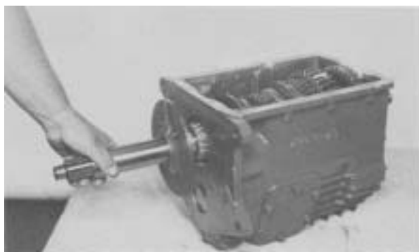
Figure 6 - Remove bearing cap.
