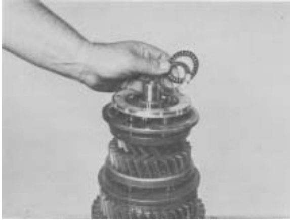
Figure 19 - Remove shift hub thrust bearing and bearing race.
