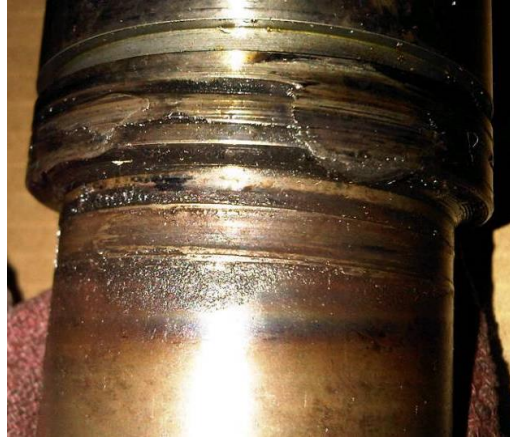
Damaged oil return threads
