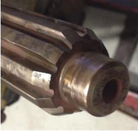
Worn input shaft pilot surface
